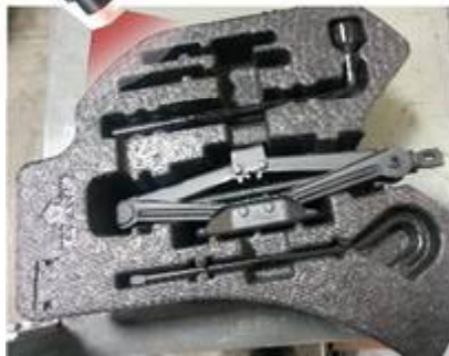
Vision detects unfilled slots in a Jack Kit
